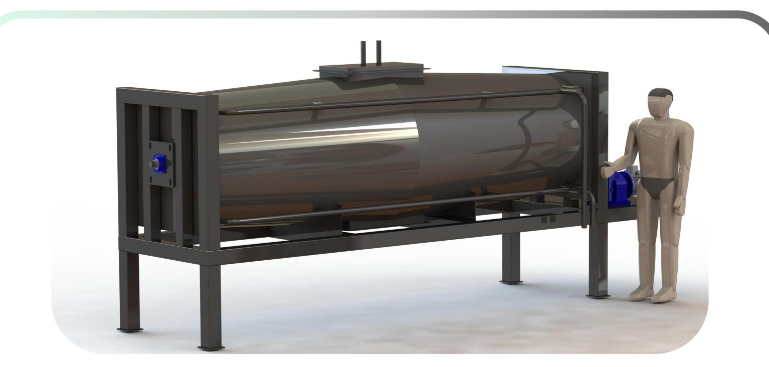
The Type B bioreactor is a horizontal cylindrical rotating reactor. It is a different approach with a different mixing logic as a key element, with all the materials being stirred as the reactor body rotates.
